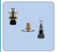
Manually operated drain valves are integrated as standard equipment in all filter bowls or filter-pressure-regulator bowls. On plastic bowls or metal bowls with sight glass a plastic drain screw is used. A metal drain screw is used on metal bowls without sight glass, but if desired it can be optionally screwed into any other bowl with female port thread in place of the plastic drain screw.
